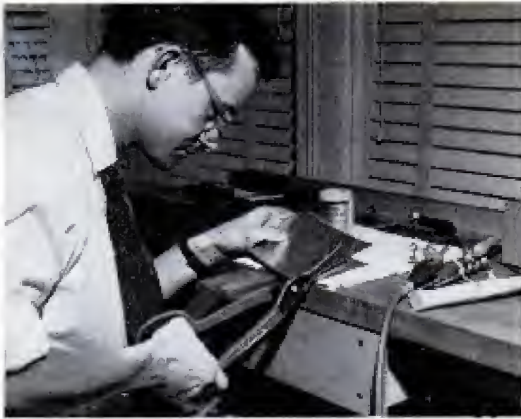
First step in making a silver ring is to snip a 1/4-inch band of silver from sheet. Cox worked as silversmith before TV
